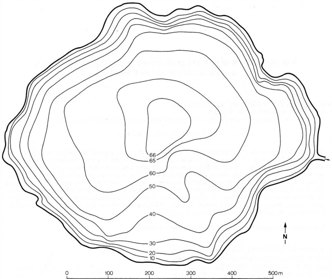
Fig. 2. Bathymetric map of Laguna de Río Cuarto. Depth isolines are given in meters.
